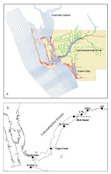
Fig. 2. The Caloosahatchee Estuary 3-D hydrodynamic model: (a) model domain; (b) monitoring stations maintained by the SFWMD.
